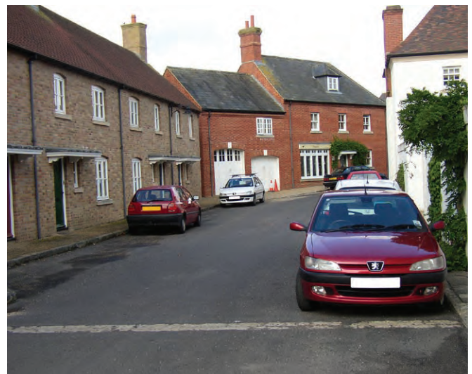
↑ The curved street design slows traffic
